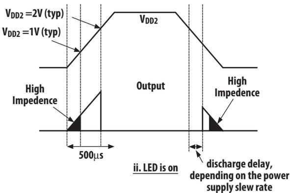
Figure 14.  $V_{DD}$  Ramp when LED is on.
