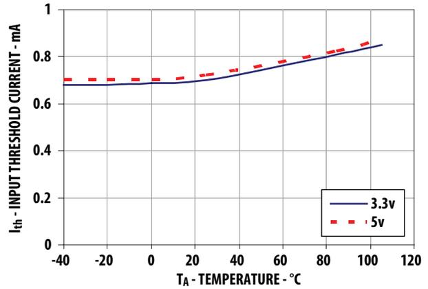
Figure 2. Typical input threshold current versus temperature.
