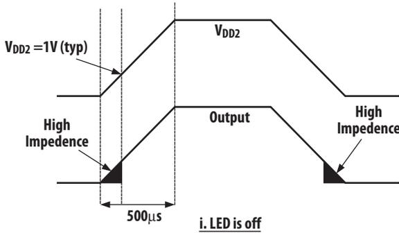
Figure 13.  $V_{DD}$  Ramp when LED is off.
